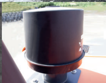
Centrifugal pre-cleaner Top Spin™ Donaldson® series
