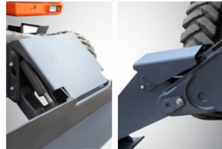
Protection covers for Dozer & Outrigger
