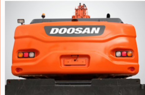
Low center of gravity designed Counter-weight
