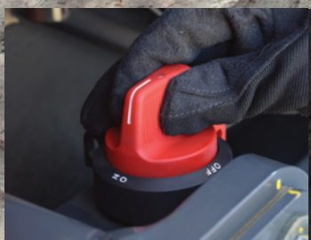
Battery cut-off switch
