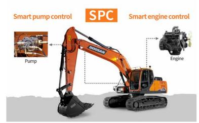
SPC is a predictive powertrain control system, which automatically identifies working mode and adjusts engine RPM to supply proper pump torque. SPC relieves the driver's workload and contributes to a fuelefficient working style. Raising the pump torque up to maximize when productivity and power is needed. Lowering the pump torque down to reduce unnecessary fuel consumption when fuel efficiency is needed.
